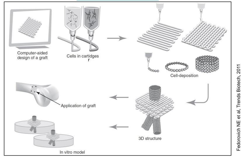
Figure 1. Organ/tissue printing using fiber deposition. Computer-assisted design of the implant is translated by the rapid prototyping machine into a layered, cell-laden hydrogel structure with defined external shape and internal morphology, for use either in an in vitro model or in vivo grafting. The availability of multiple printing heads, each containing a specific cell type or hydrogel, enables printing of heterogeneous constructs.
