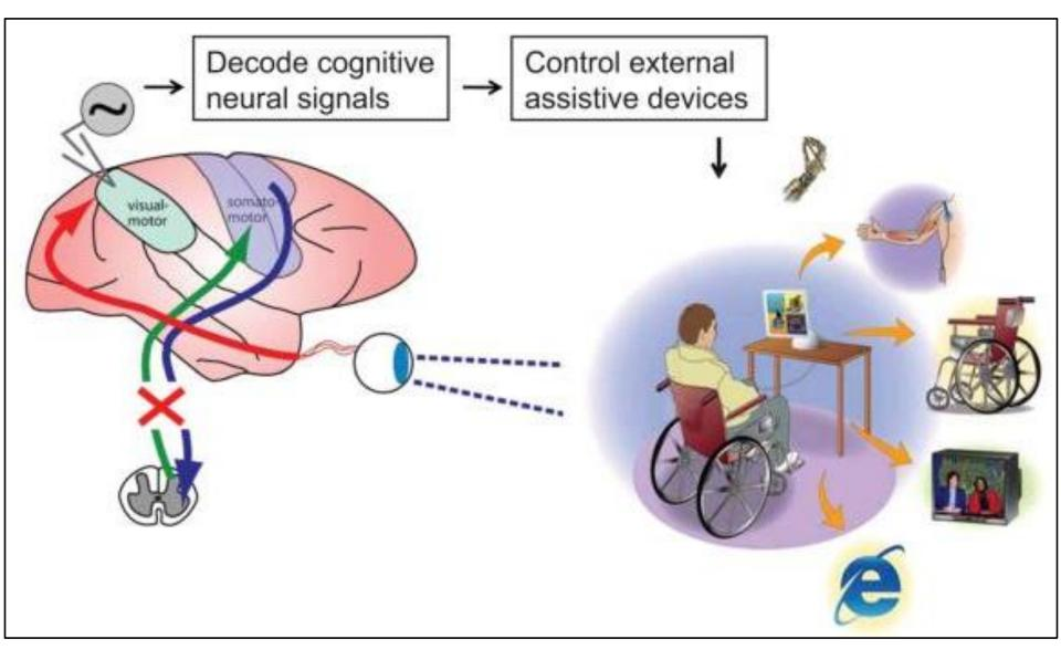
Schematic representation of a cognitive neural prosthetic. In this example, the patient has a lesion of the spinal cord, represented by the red X on the brain drawing on the left. The patient can still see the goal of a movement and can plan the movement, but cannot execute it.
