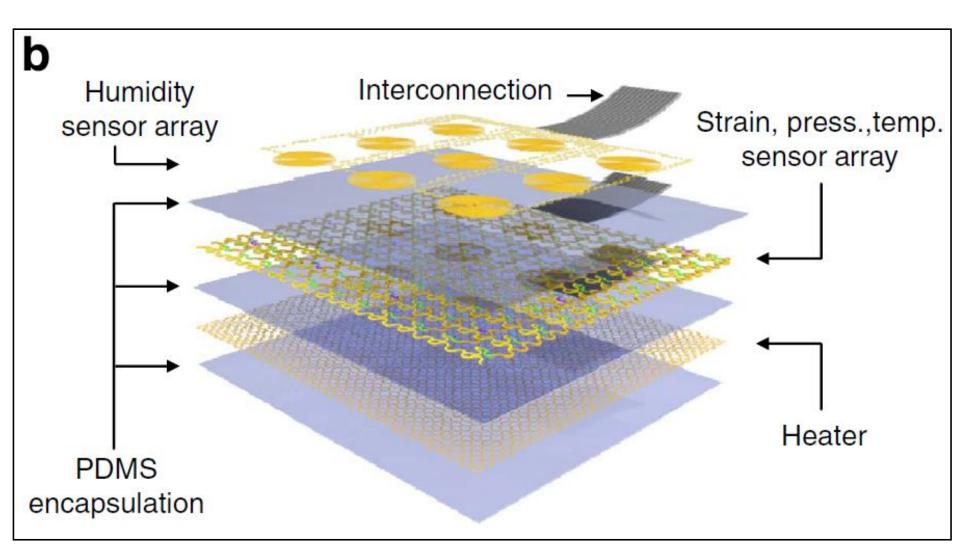
(b) An exploded view of the artificial skin comprised of six stacked layers. Interconnected wires of each layer relay signals to external instruments.
