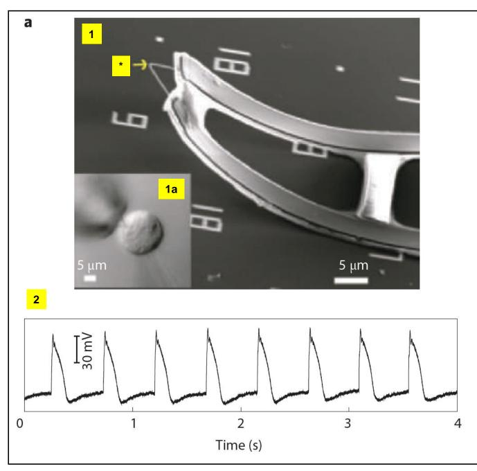
Figure 4 | Nanodevices in tissue engineering. a, Threedimensional, freestanding nanowire transistor probe for electrical recording. The probe is composed of a kinked nanowire (yellow arrow) and a flexible substrate material. The device is used to penetrate the membrane of living cells (inset) and measure intracellular signals (lower panel).
