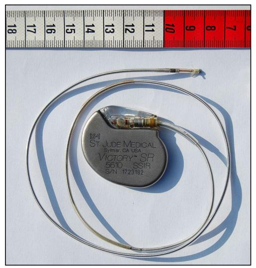
A **pacemaker** is a small device that's placed in the chest or abdomen to help control abnormal heart rhythms. This device uses low-energy electrical pulses to prompt the heart to beat at a normal rate. **Pacemakers** are used to **treat arrhythmias**. Arrhythmias are problems with the rate or rhythm of the heartbeat.
